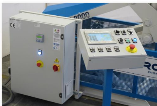
■ Available Voltages: 400V - 50/60Hz CE 480V - 60Hz UL complied 600V - 60Hz CSA complied
