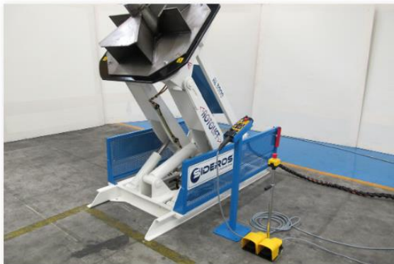
■ Remote pushbutton panel and foot pedal to ease movement control
