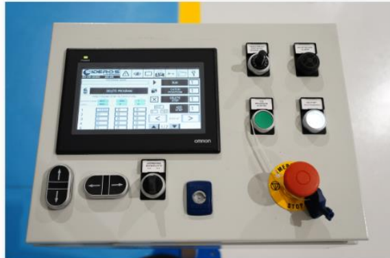
■ Touch screen HMI with Teaching System for automatic programming of movement steps
